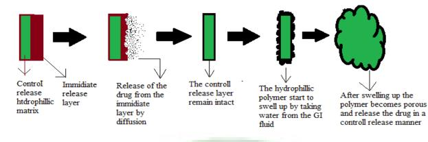
Figure 3: DUREDAS technology consists of control release and immediate release layer.
