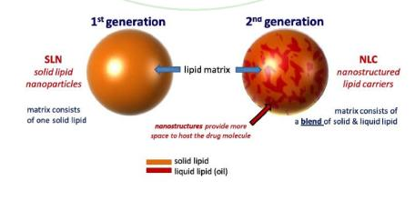
Figure 4: Difference between an SLN and an NLC particle matrix structure
