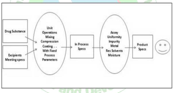
Figure1: Simplified quality control diagram using QbT
