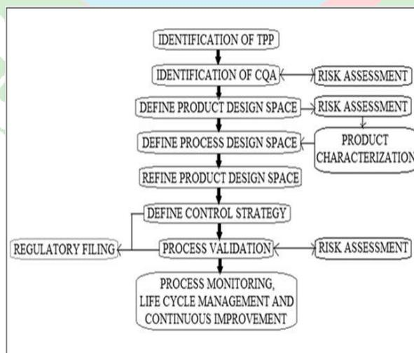
**Figure 3: Key Steps In Implementation of QbD for a Pharmaceutical Product TPP-Target Product Profile, CQA-Critical Quality Attributes**
