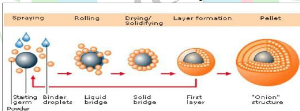
Figure 2: Principle of powder layering process
