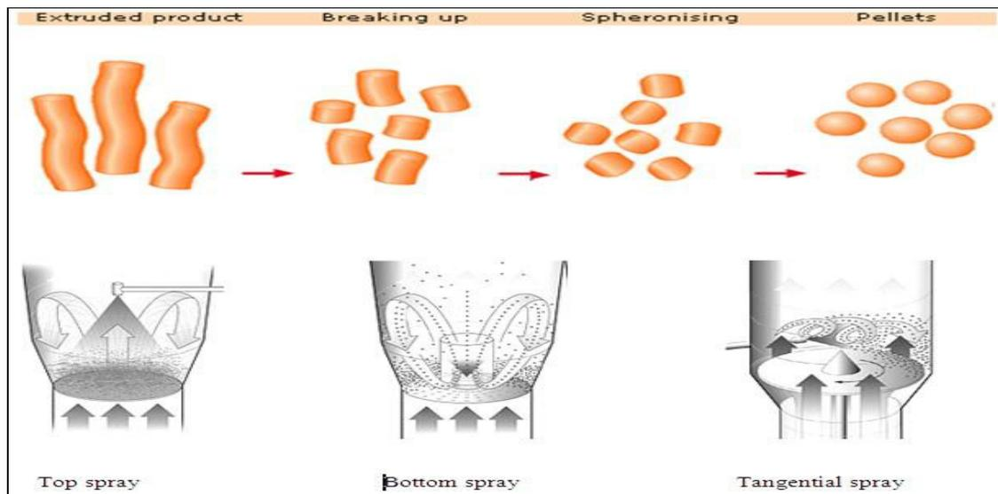
Figure 4: Schematic representation of Different pellets formation stages during spheronization
