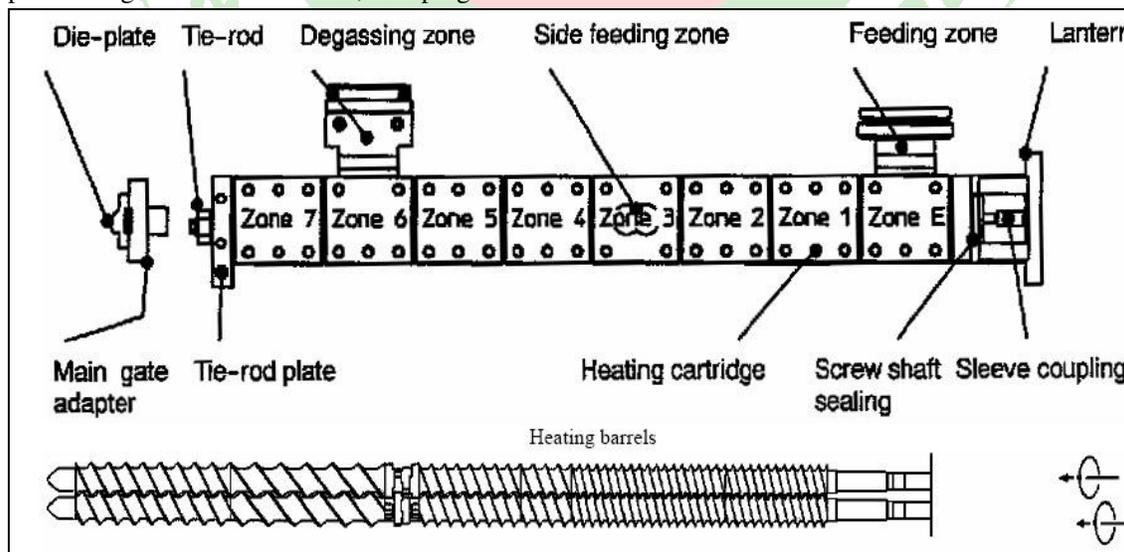
Figure 5: Heating barrels and co-rotating screws for hot-melt extruder
