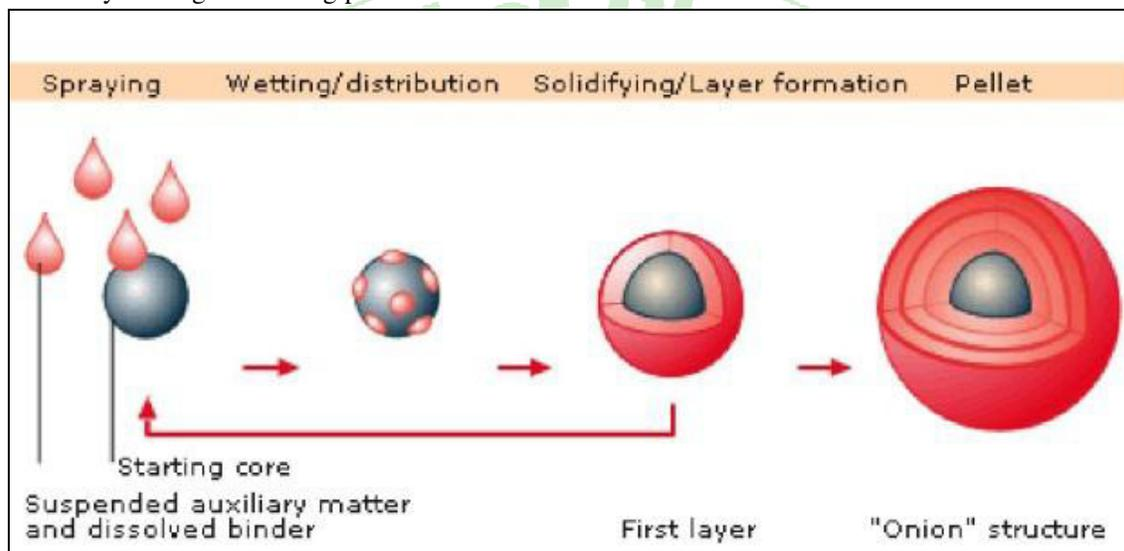
Figure 3: Principle of solution and suspension layering process
