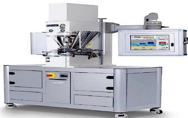
Figure: 7 Bi-layer Tablet Press with Displacement Monitoring (31)
