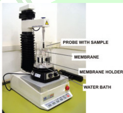
Figure 7: Bioadhesion test using the texture analyzer
