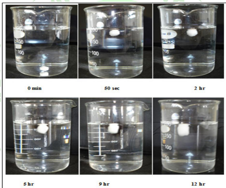
**Figure 6: Floating Lag Time of Quetiapine Hemifumarate Floating Matrix Tablet F1**
