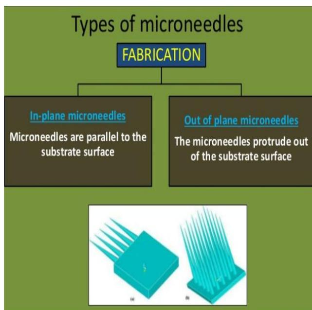
Figure 1: Classification on the basis of fabrication.
